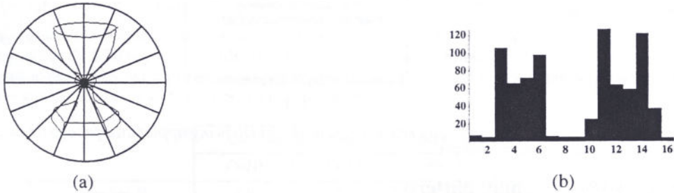
Figure 6 : Graphical representation of the circular histogram. (a) The centre of gravity of the watermark is used as the middle point to compute the circular histogram. (b) Representation of the histogram computed from the figure (a).
